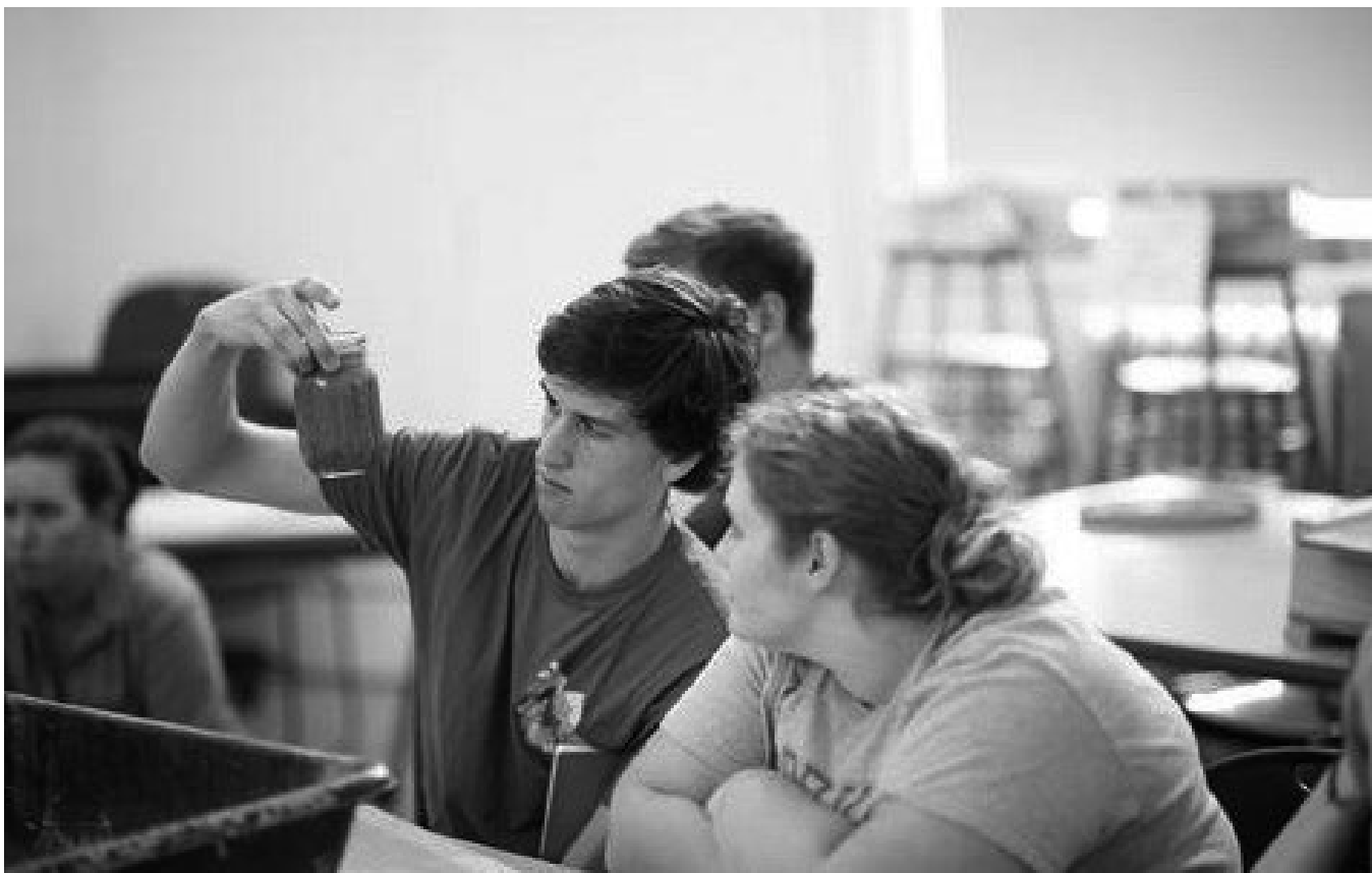
Figure 4: Students conducting the shake test to assess particle composition percentages within a specific soil sample.
