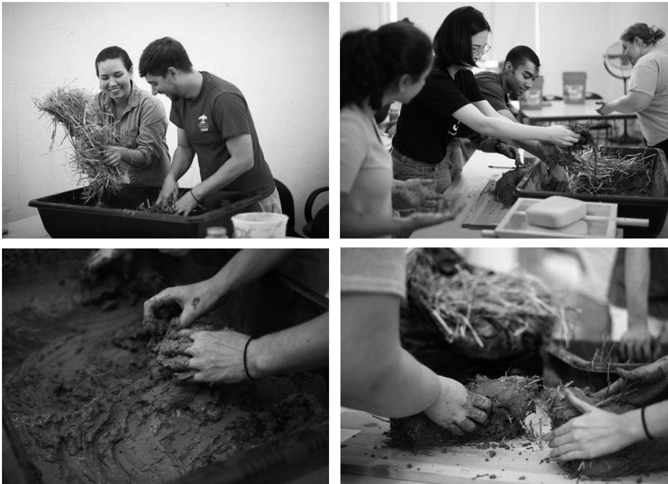
Figure 3: Students designing optimal earth- and bio-based mixtures at the course's materials laboratory.
